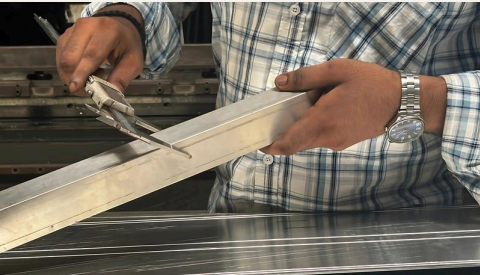
Marking a stainless steel section for cutting
