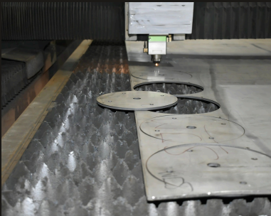
CNC laser cutting circular profiles from sheet metal
