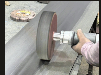
Polishing a stainless steel surface with a flap wheel
