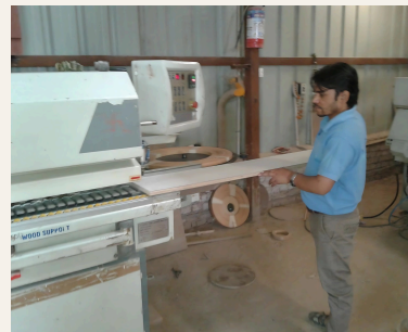
Feeding a panel through the edge-banding machine
