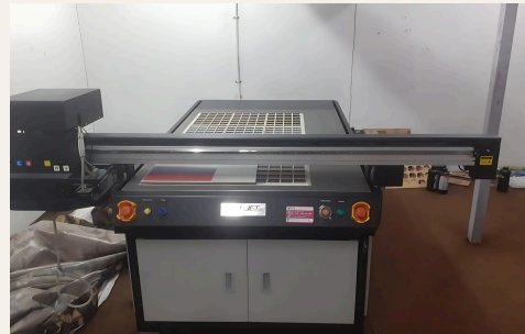
UV flatbed printer for surface printing
