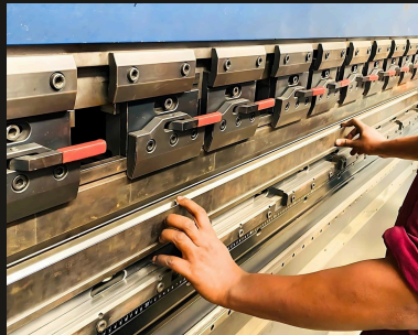
Setting tooling on the CNC bending machine
