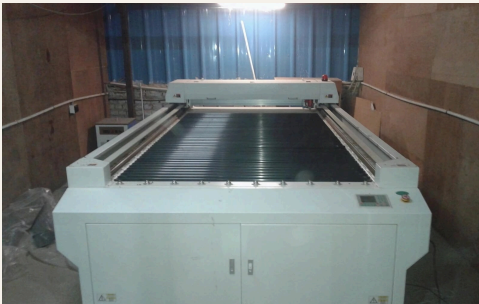
Large-format laser cutting and engraving machine
