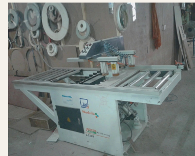
Multi-spindle boring machine for panel drilling
