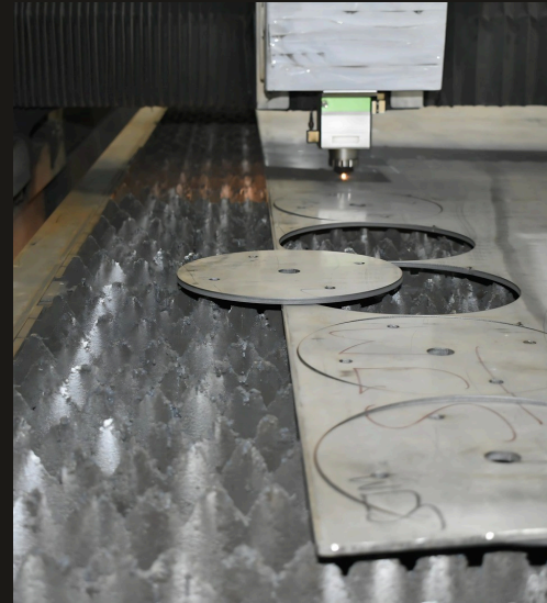
CNC laser cutting circular profiles from sheet metal
