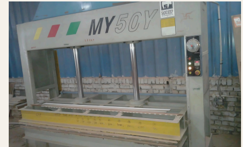
Hydraulic press for laminating panels
