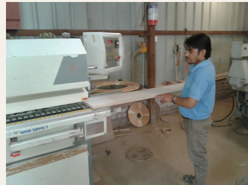
Feeding a panel through the edge-banding machine
