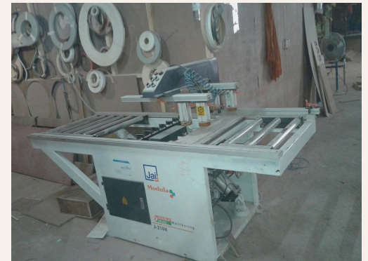
Multi-spindle boring machine for panel drilling
