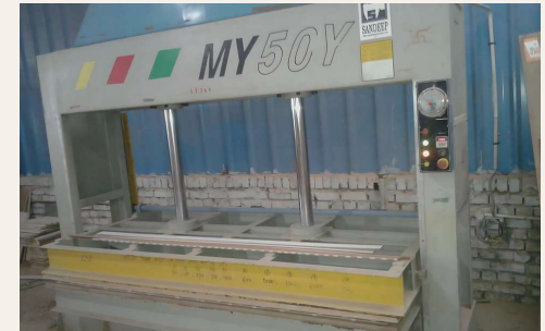
Hydraulic press for laminating panels
