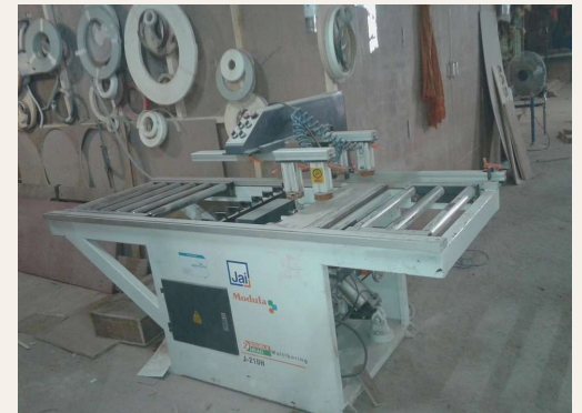
Multi-spindle boring machine for panel drilling
