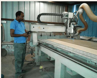
CNC router machining a panel
