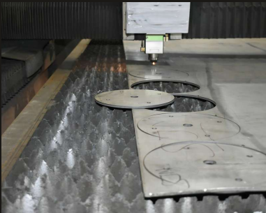
CNC laser cutting circular profiles from sheet metal
