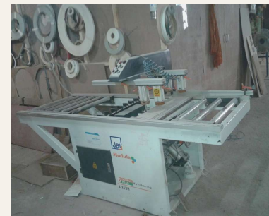
Multi-spindle boring machine for panel drilling
