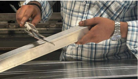
Marking a stainless steel section for cutting
