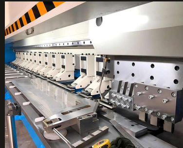
CNC V-grooving machine for sharp-edged folds in cladding and profiles
