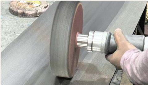
Polishing a stainless steel surface with a flap wheel
