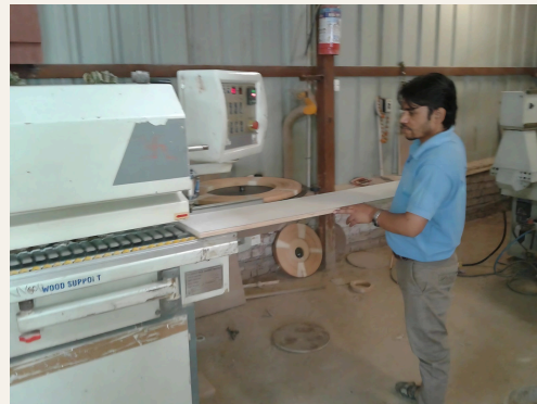
Feeding a panel through the edge-banding machine
