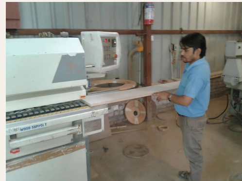
Feeding a panel through the edge-banding machine
