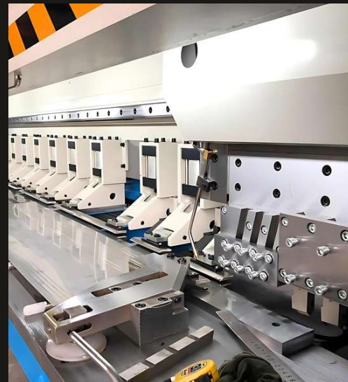
CNC V-grooving machine for sharp-edged folds in cladding and profiles
