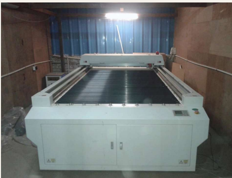
Large-format laser cutting and engraving machine
