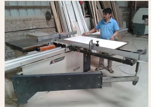
Sizing a laminated panel on the panel saw
