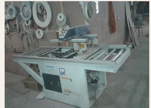
Multi-spindle boring machine for panel drilling
