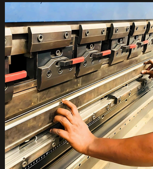
Setting tooling on the CNC bending machine
