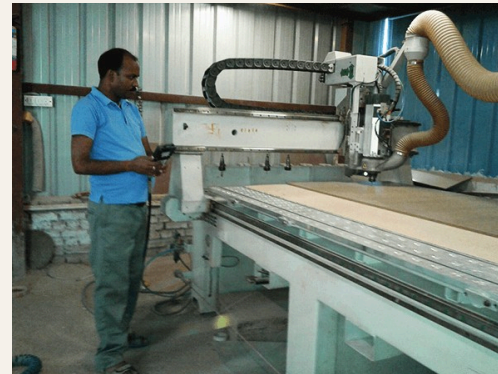
CNC router machining a panel
