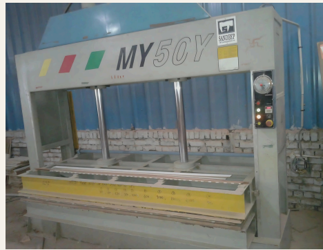
Hydraulic press for laminating panels
