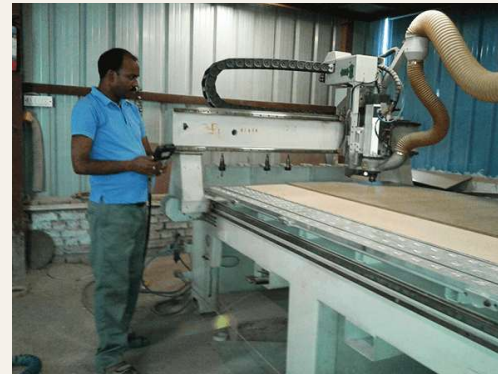
CNC router machining a panel
