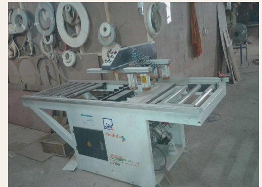
Multi-spindle boring machine for panel drilling
