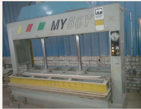
Hydraulic press for laminating panels
